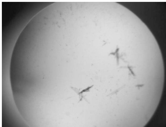
Figure 1 The crystals of NlaX MTase used for diffraction studies. Crystal dimensions are 0.05 × 0.07 × 0.15 mm.
